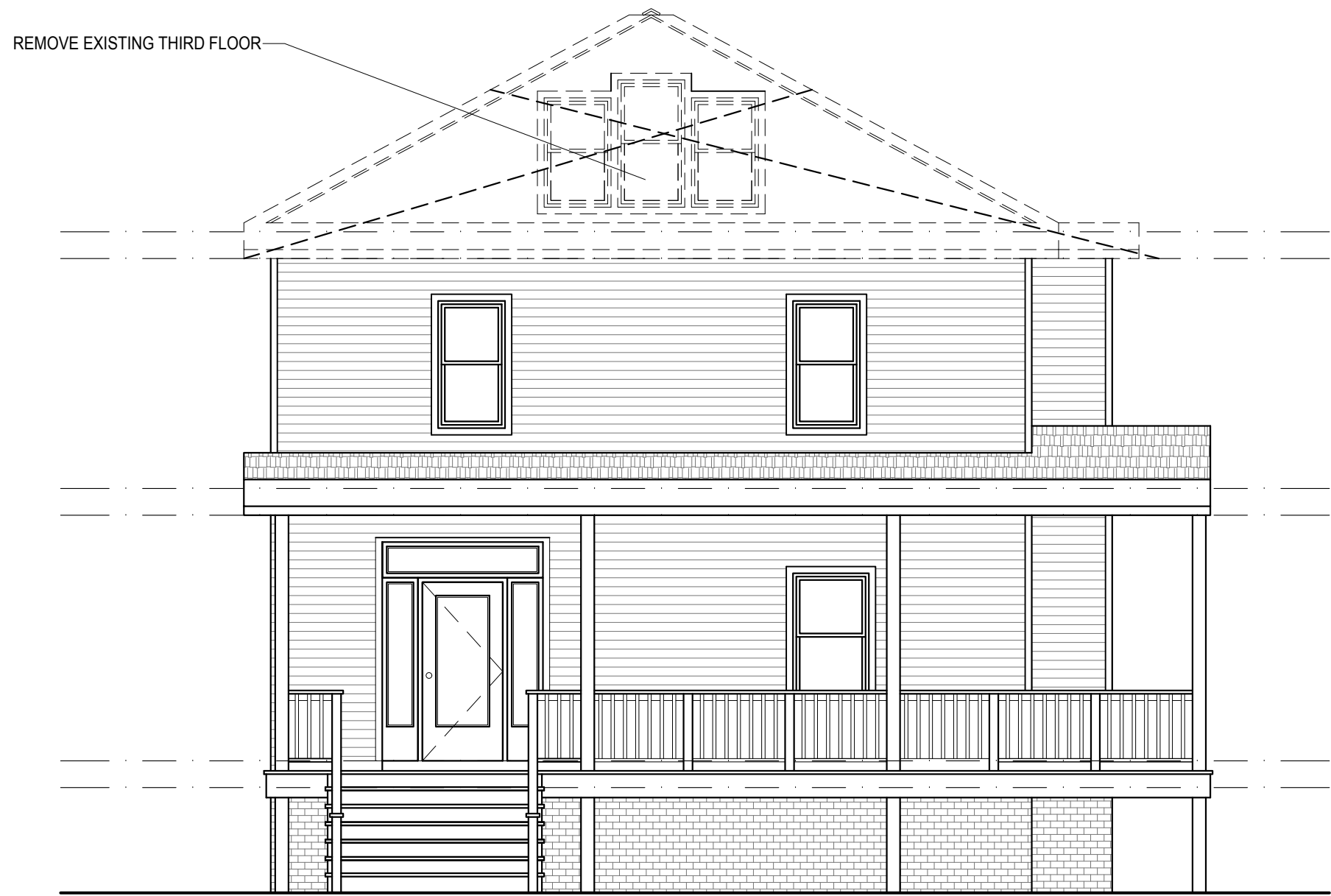
1 DEMO FRONT ELEVATION SCALE: 3/16" = 1'-0"
